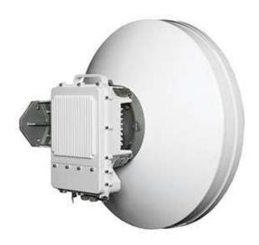
The SkyWay-EB3 95GHz ULL W-Band PTP Link is a modified version of the EB 70/80GHz ULL PTP links. The channel plan is designed to comply with the FCC 95GHz regulations for a fully symmetric 1Gbps operation using 700MHz BW. The latency figure for each pass is drastically reduced to 100ns, best-in-class for millimeter systems using less than 1GHz BW.
