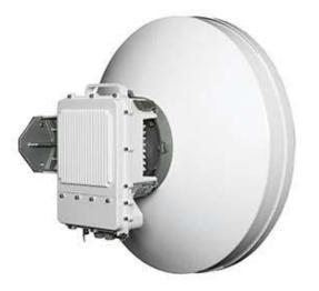
The SkyWay-EB 95GHz ULL W-Band PTP Link is a modified version of to the EB 70/80GHz ULL PTP links. The channel plan is designed to comply with the FCC 95GHz regulations for a fully symmetric 1Gbps operation using 500MHz BW. The latency figure for each pass is 400ns.
